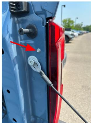
Figure 5. Tail Lamp Removal
